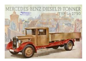
The robust and compacted Mercedes-Benz Truck LO 2750 with its fuel-efficient 65-hp diesel engine was a popular transport vehicle for small- and medium-sized enterprises during its heyday. Owing to its big loading space and a carrying capacity up to 2 ¾ tons that it offered, the truck was capable of fulfilling nearly all haulage-related tasks excellently.
